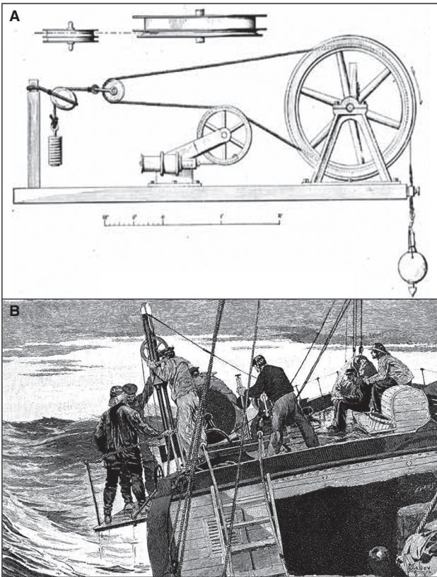
**Fig. 2** (A) Diagram of the original version of the piano-wire sounding machine or Thompson Sounding Machine invented by Sir William Thomson (later Lord Kelvin) in 1872. (B) “The United States Fish Commission” by Richard Rathbun. Century Magazine, Vol. 43, issue 5. 1892. “Sounding the abyss with piano-wire.” This image is among the most realistic representations of sounding with the Sigsbee Sounding Machine.
