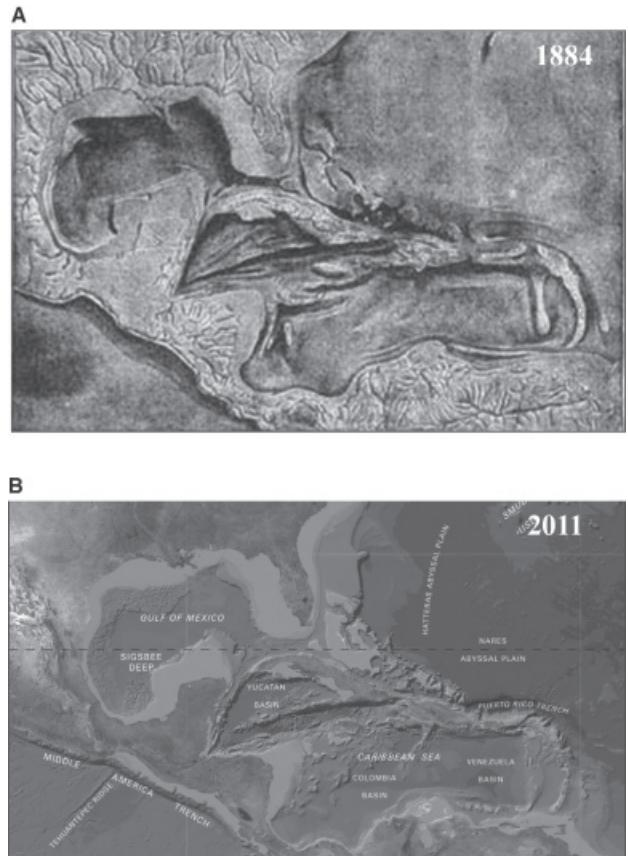
**Fig. 3** Early mapping efforts along coastal margins were quite accurate, particularly as shown in (A) the first 3D rendition of ocean bathymetry of the Gulf of Mexico and Caribbean Sea produced in 1884 from the Blake soundings. (B) Same region highlighted from current bathymetric maps has many of the same features.
